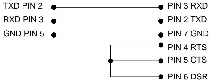
Printer (DSUB 9 plug)      PC (DSUB 9 socket)
