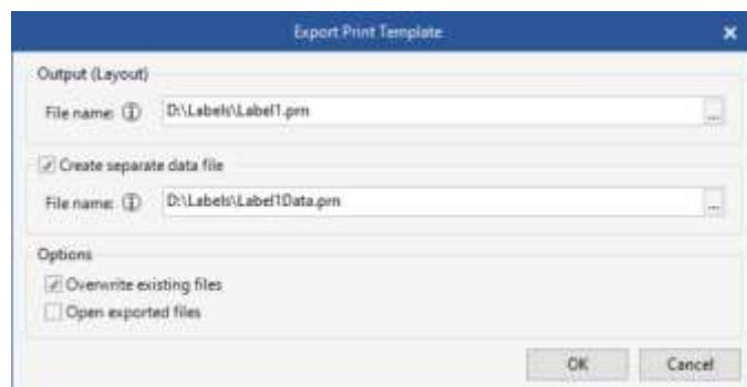
The option **Create separate data file** must be selected, otherwise the line (SOH)**FBC---r-----(ETB)** is included in the print file, which would immediately release a print procedure.
