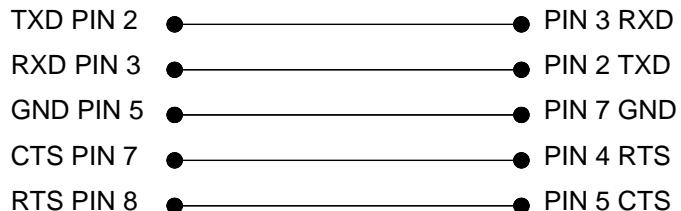
Printer (DSUB 9 plug)      PC (DSUB 9 socket)
