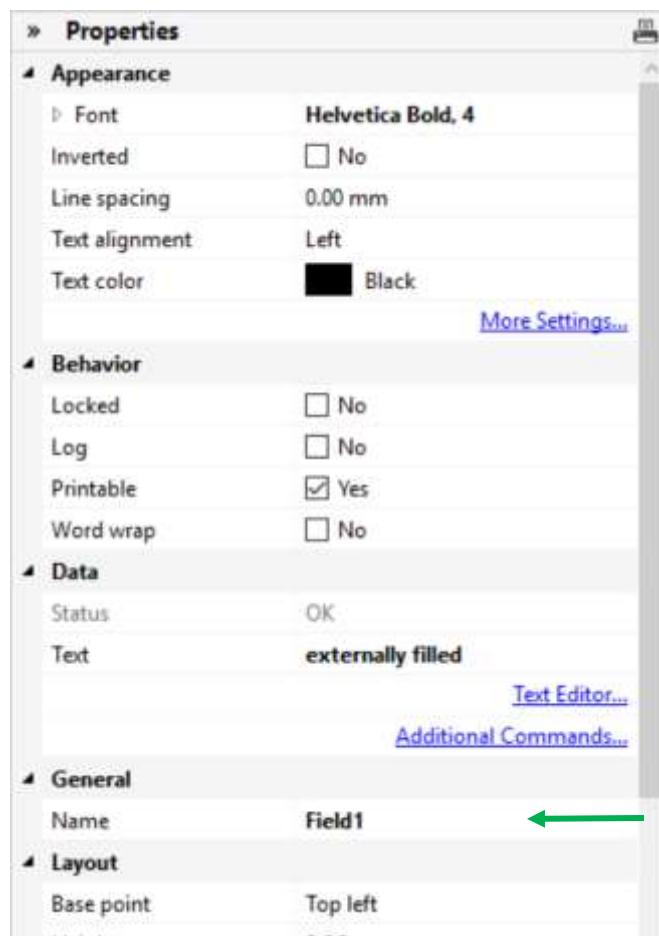
The desired field name (Field1) is entered in the properties of the text field.
