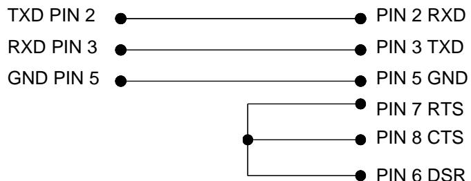
**Hardware Handshake**      Printer (DSUB 9 plug)      PC (DSUB 25 socket)
