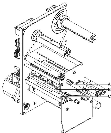
A soiled print roller can lead to a reduced print quality and can affect the transport of material.
