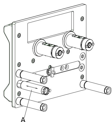
A soiled ribbon roller can lead to reduced print quality and can affect transport of material.
