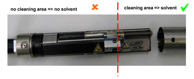
Especially the area around the oscillator connection must not be flushed with solvent. Otherwise solvent could penetrate inside the oscillator or the connector and could cause damages or mal functions.
